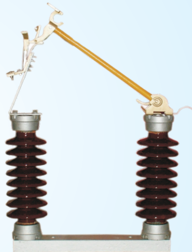
22/33 KV Outdoor Expulsion type Drop Out Fuse Solidcore Insulators with channel Base. Test as per IS-9385/1983
