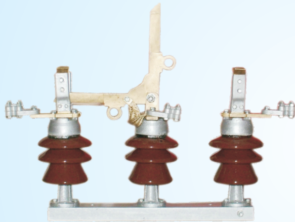
11/22/33 KV Outdoor Three insulator per pole tilting type, Gang Operated Single Phase Switch Suitable for horizontal / vertical mounting. Test as per IS-9920 / 1985
