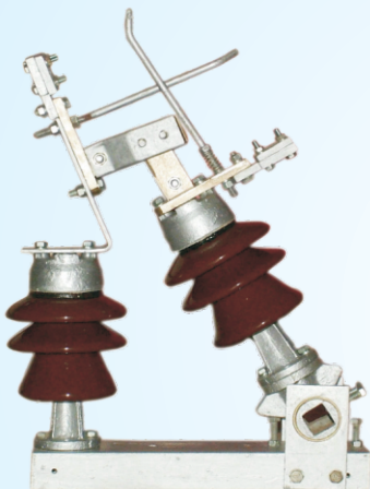
11/22/33 KV Outdoor triple pole Two insulator per pole tilting type, Gang Operated Air Break Switch Suitable for horizontal / vertical mounting with complete operating mechanism. Test as per IS-9920 / 1985
